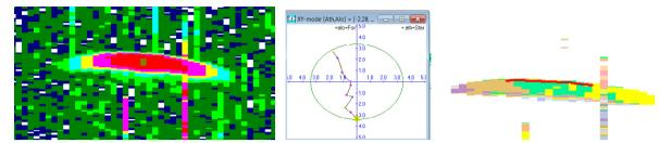
**Fig. 3.** Echo from Target *ID* nr 6, Table 5, believed to originate from *P. gladius*. Left: Echogram with fish trace and background noise, the *x*-axis is ping and the colors indicate a very strong echo in the center weakening to the sides. Center: Position diagram showing the boat/fish passage. Left: sample angle echogram showing the athwart ship sample angles interpreted as colors. Yellow = 1, green = -1, orange = -2 deg.
